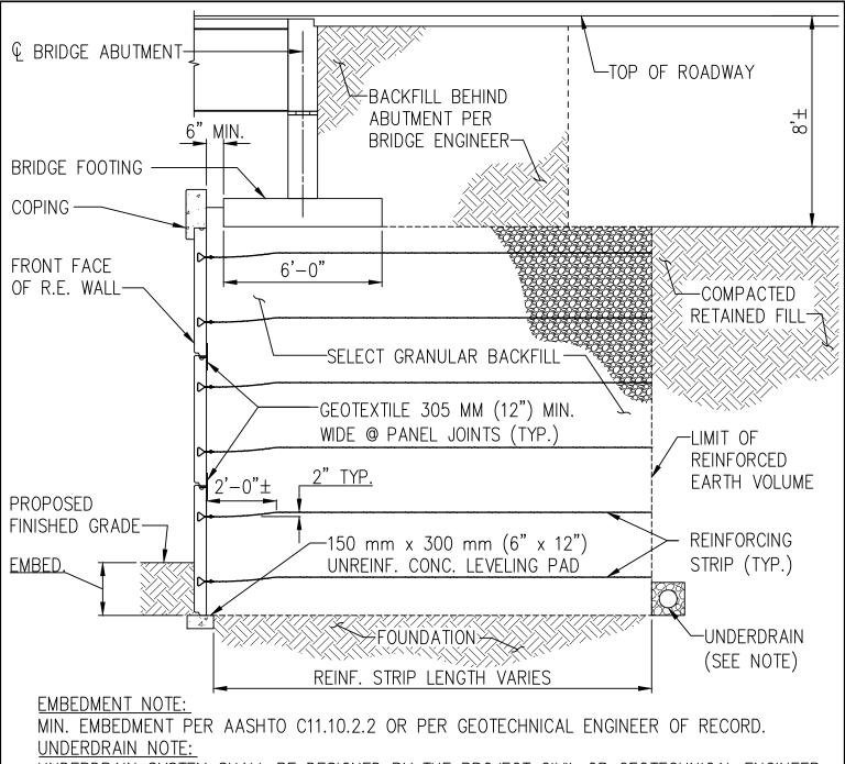
UNDERDRAIN SYSTEM SHALL BE DESIGNED BY THE PROJECT CIVIL OR GEOTECHNICAL ENGINEER OF RECORD BASED ON SITE CONDITIONS. UNDERDRAIN SHALL BE SLOPED TO DRAIN AND OUTLET TO ADJACENT DRAINAGE STRUCTURES OR BEYOND THE LIMITS OF THE MSE WALL. FOUNDATION NOTE:
