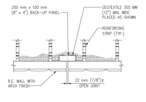
PARTIAL PLAN - SLIP JOINT DETAIL SCALE: 3/4" = 1'- 0"
