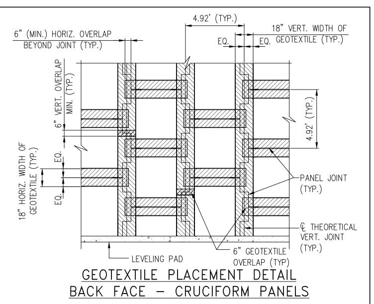
PROPER INSTALLATION OF GEOTEXTILE AT PANEL JOINTS IS IMPERATIVE IN PREVENTING LOSS OF BACKFILL MATERIAL.
