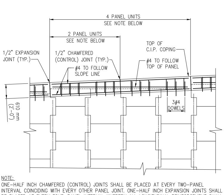
INTERVAL COINCIDING WITH EVERY OTHER PANEL JOINT. ONE-HALF INCH EXPANSION JOINTS SHALL BE PLACED AT EVERY FOUR-PANEL INTERVAL WHEREBY ALL LONGITUDINAL REINFORCEMENT SHALL BE FIELD CUT TWO INCHES (2") SHORT OF EACH SIDE OF THE EXPANSION JOINTS.
