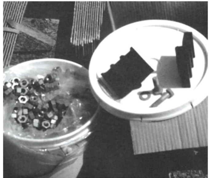
Figure 10: Fasteners and bearing pads.
